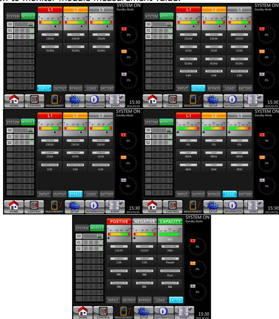
Figure 4-10 Module Measurement Screens
